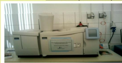
GC-MS used to additionally check the mass concentration of alcohol standard solution obtained by gravimetric method
