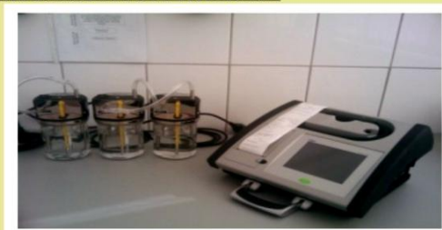
Mark II A thermo-controlled flasks, and Alcotest 9510 ethylometer, both produced by Dräger Safety AG & Co, KGaA, Germany
